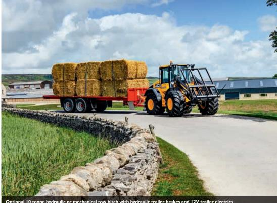
Optional 10 tonne hydraulic or mechanical tow hitch with hydraulic trailer brakes and 12V trailer electrics further improve versatility.
